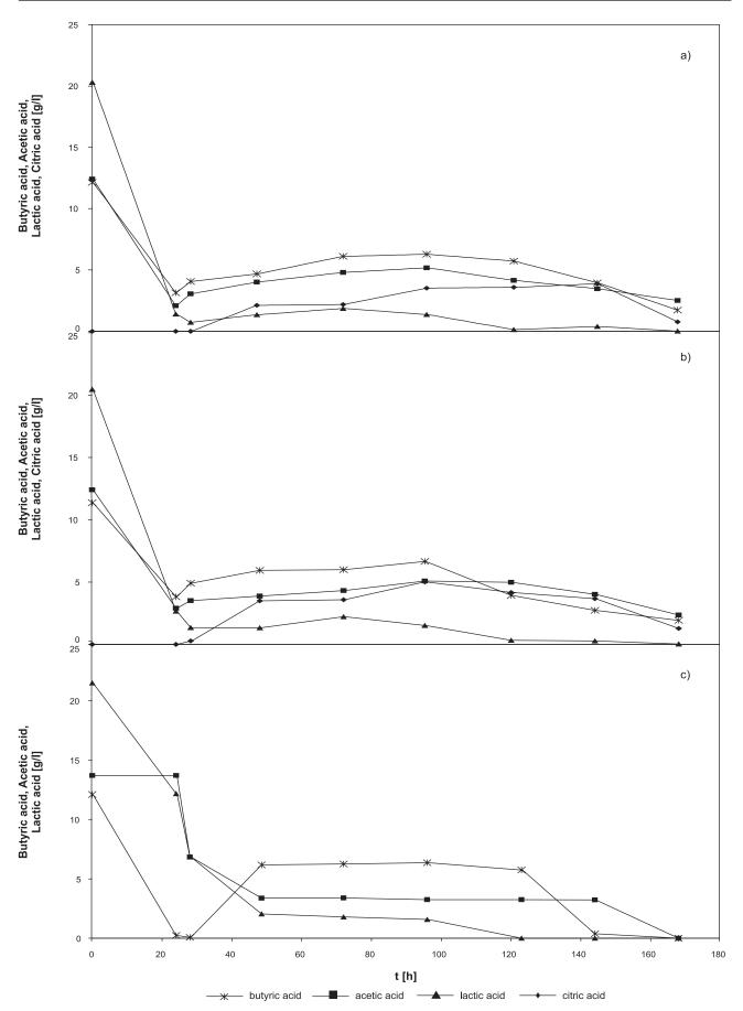
Fig. 6. Variations in the content of the organic acids chosen during biodegradation in the STR. a) 550 rpm, no pH control, b) 900 rpm, no pH control, c) 900 rpm, pH = 8.35.
