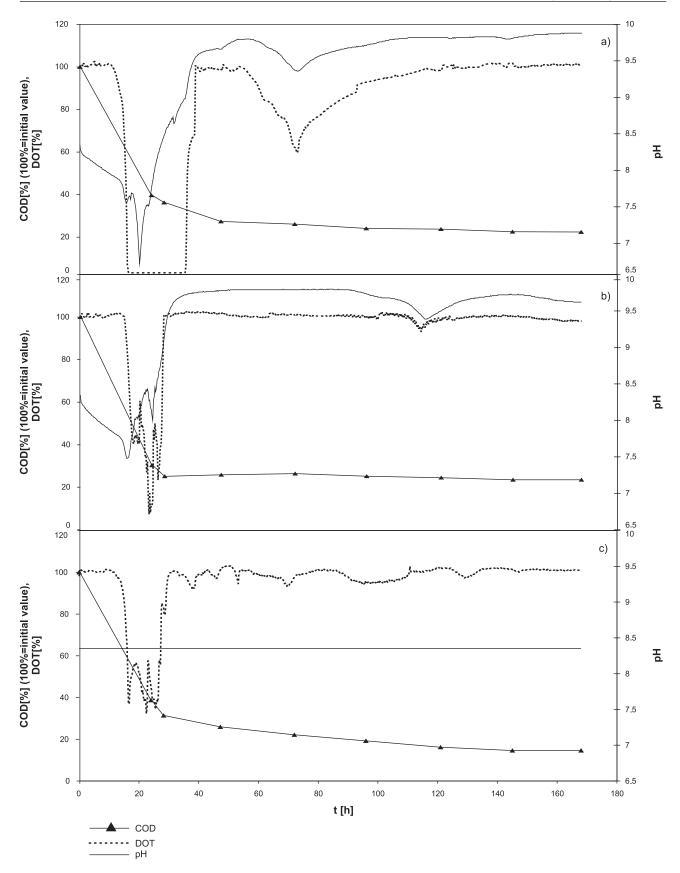
Fig. 5. Variations in the parameters chosen during the biodegradation of vinasse in the STR. a) 550 rpm, no pH control, b) 900 rpm, no pH control, c) 900 rpm, pH = 8.35.
