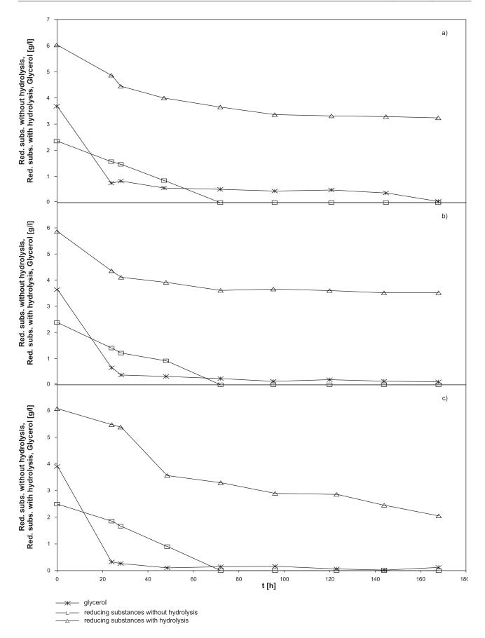
Fig. 7. Variations in the concentration of glycerol and the reducing substances during biodegradation of vinasse in the STR. a) 550 rpm, no pH control, b) 900 rpm, no pH control, c) 900 rpm, pH = 8.35.
